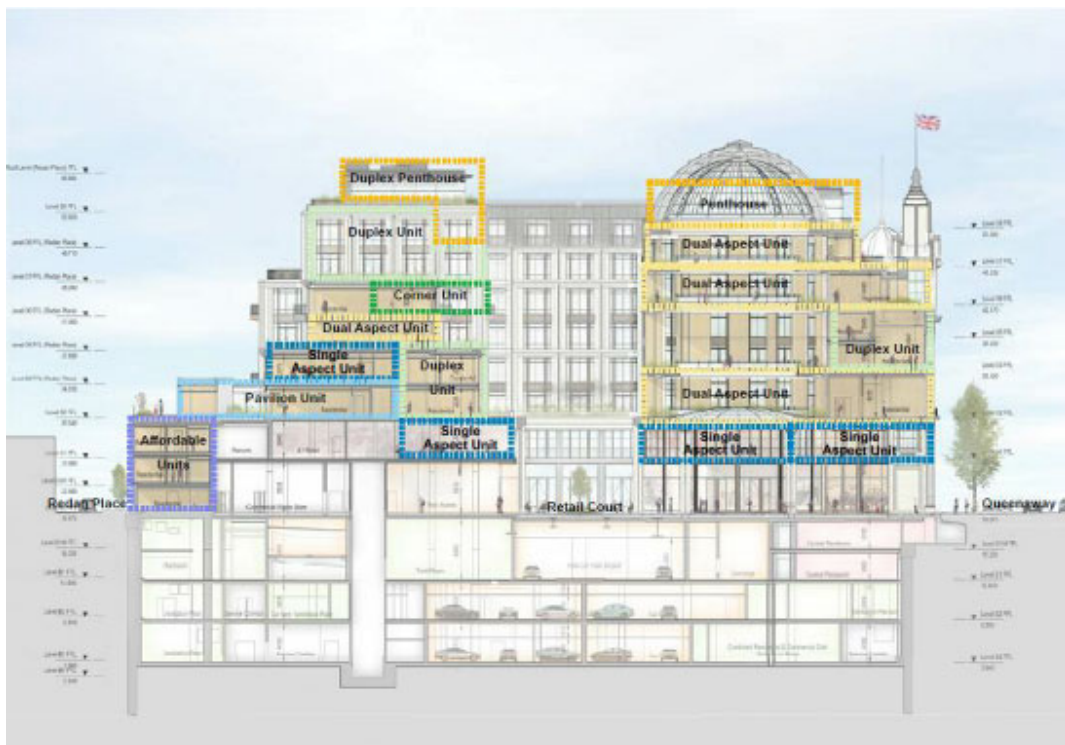
As approved section (top) and as proposed section (bottom) showing reduction in basement depth.
